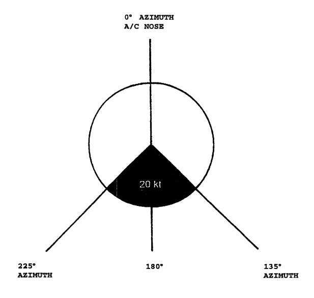
Figure 1. REARWARD AIRSPEED LIMITATION DIAGRAM
